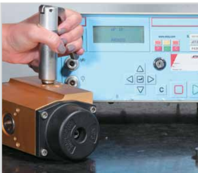
Leack test machine. For pneumatic rotary actuators.
