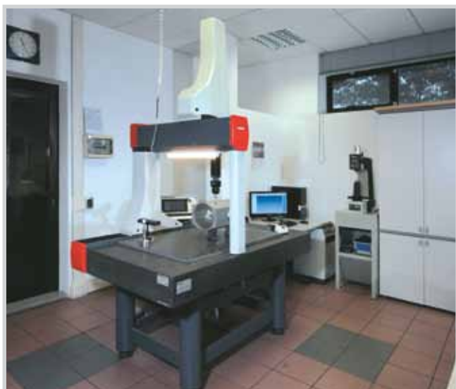
Coordinate Measuring Machine. CMM
