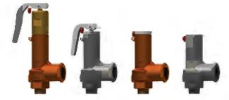
THE VALVE WORKS AS AN AUTOMATIC PRESSURE RELEASING REGULATOR ACTIVATED BY THE STATIC PRESSURE EXISTING AT THE ENTRANCE TO THE VALVE AND IS CHARACTERIZED BY ITS ABILITY TO OPEN INSTANTLY AND TOTALLY. DESIGN IN ACCORDANCE WITH "ASME CODE SECTION VIII". MATERIALS ACCORDING ASME CODE SECTION II AND ASTM. CONNECTIONS ACCORDING ASME B1.20.1 STANDARD.
